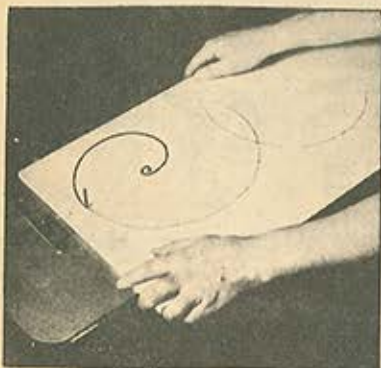
Figure 16--Cutting toward the operator. Unnecessary to turn the work.
