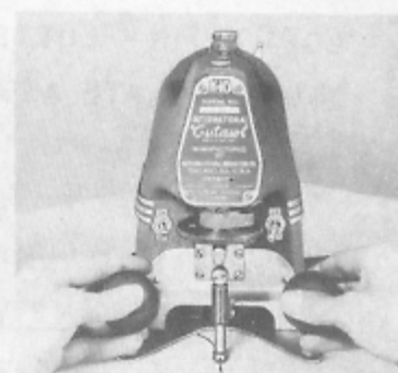
Figure 13--- Cutawl cutting away from the operator.
