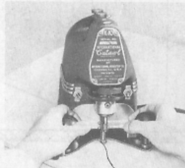
Figure 11---Cutawl cutting toward the operator. neither work nor Cutawl is turned.
