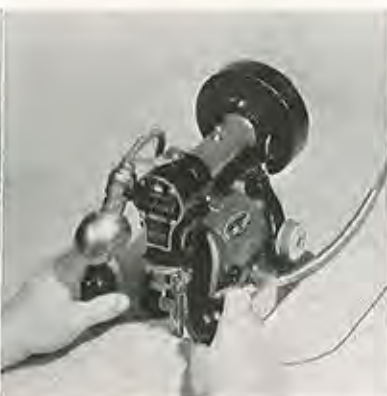
Figure 7—K9 Cutawl cutting toward the operator's left. The cutting mechanism alone does the turning
