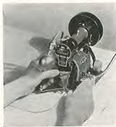
Figure 5—K9 Cutawl starting a cut using a chisel
