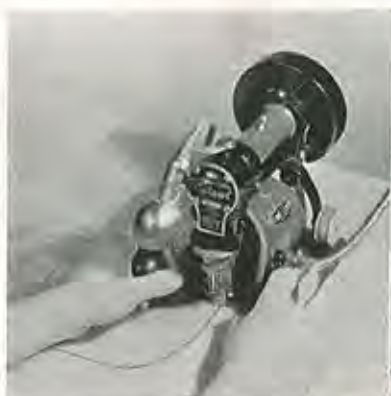
Figure 6—K9 Cutawl cutting toward the operator. Neither work nor Cutawl is turned
