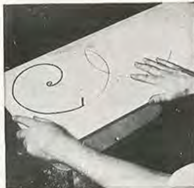
Figure 15—Cutting to the operator's right. The saw does the turning
